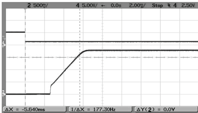
On/Off Enable Delay (Vin=12V, Vout=1.8V, Iout=6A, Load=0) Trace 4=Enable, Trace2=Vout
