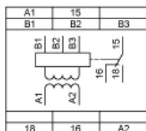
A1- Supply voltage Electrodes (see table below)
