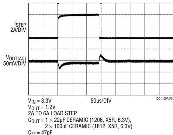
Figure 4. Measured Load Transient Response (4A Step, 25% to 75%)
