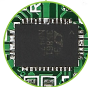
Figure 5-2: power management and battery charger IC
