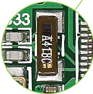
Figure 6-1: 32.768 kHz crystal oscillator module (X2)
