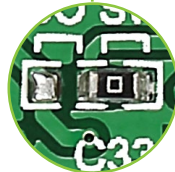
Figure 5-1: zero-ohm J1 jumper
