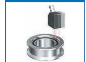
Measuring Depth of O-Ring Insertion
