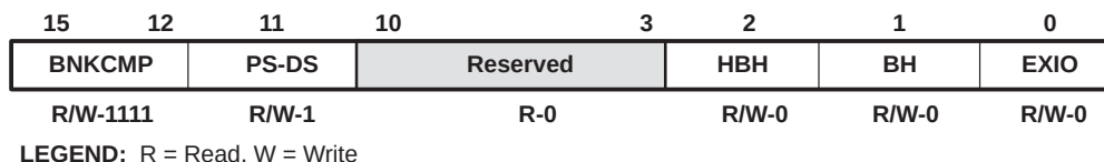
Figure 6. Bank-Switching Control Register (BSCR), MMR Address 0029h
