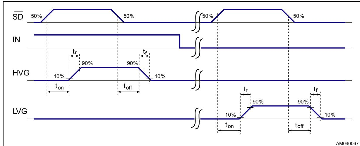
**Figure 4. IN timings and deadtime**
