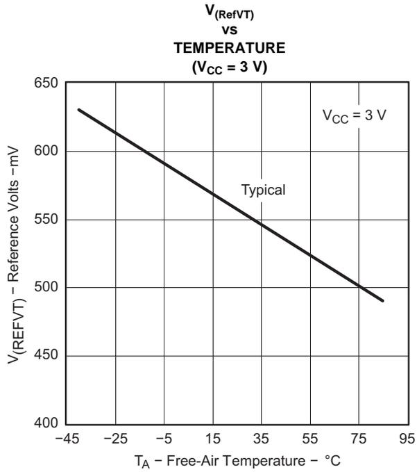
Figure 1. V<sub>(RefVT)</sub> vs Temperature, V<sub>CC</sub> = 3 V
