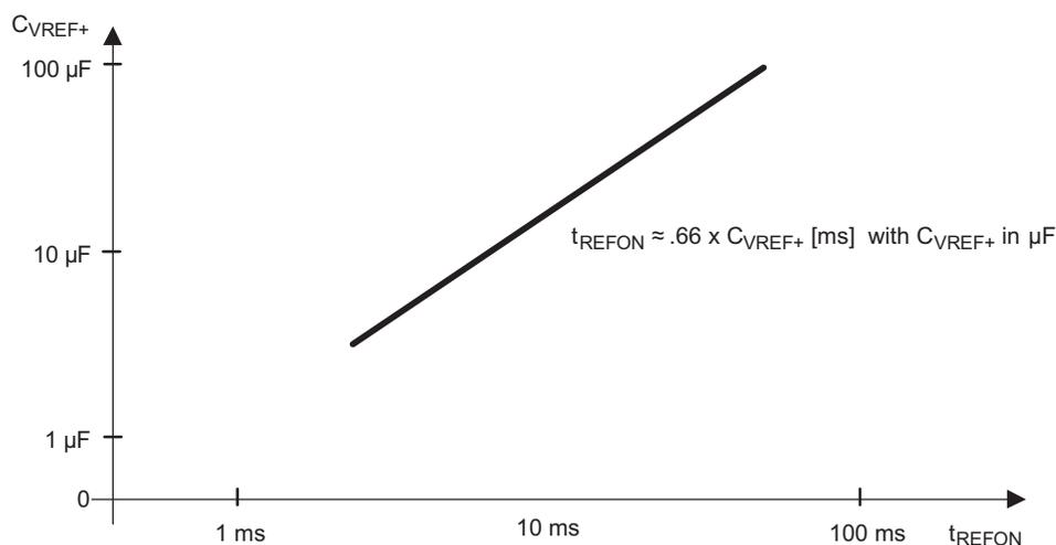
Figure 39. Typical Settling Time of Internal Reference t<sub>REFON</sub> vs External Capacitor on V<sub>REF+</sub>
