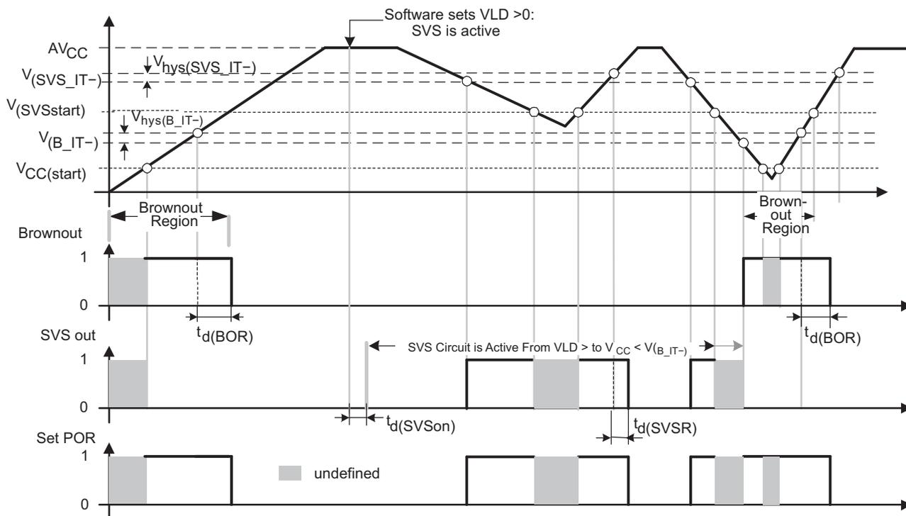
Figure 12. SVS Reset (SVSR) vs Supply Voltage
