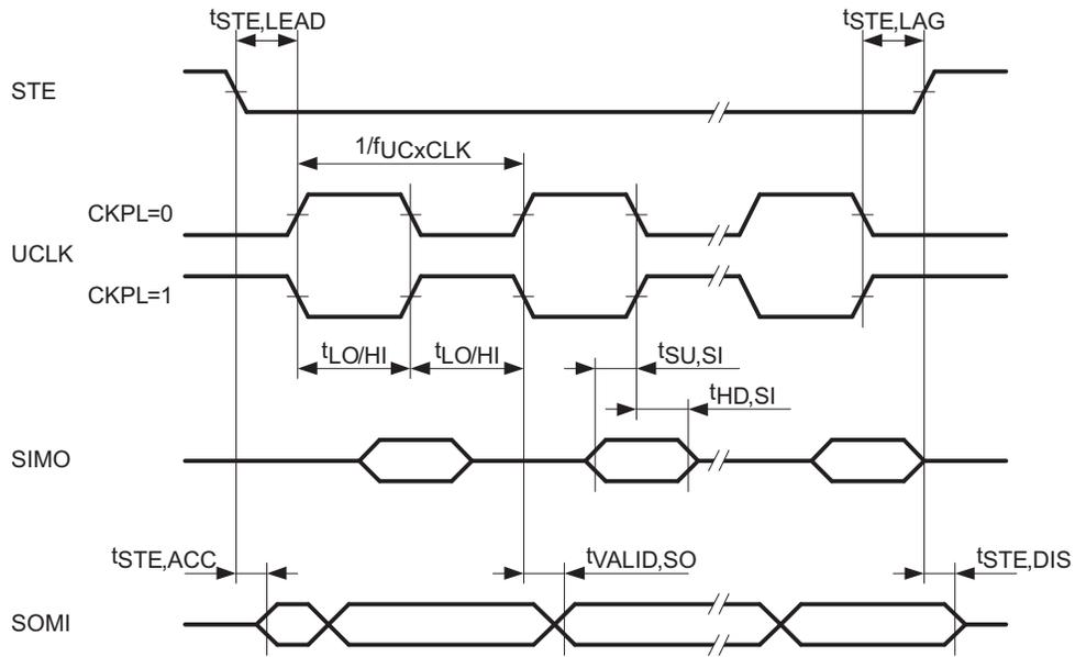
Figure 29. SPI Slave Mode, CKPH = 0
