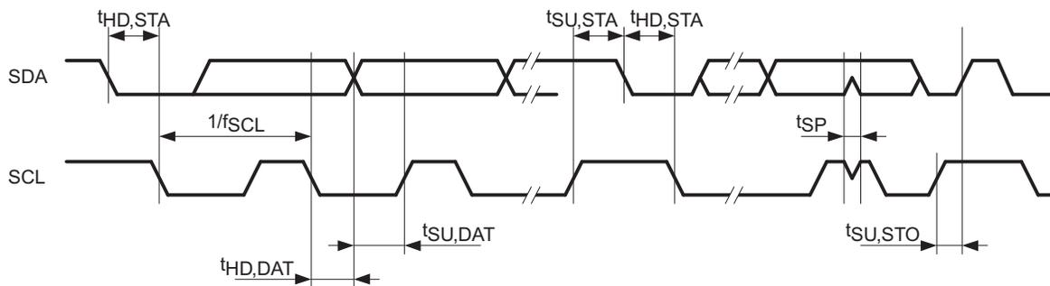
Figure 31. I<sup>2</sup>C Mode Timing
