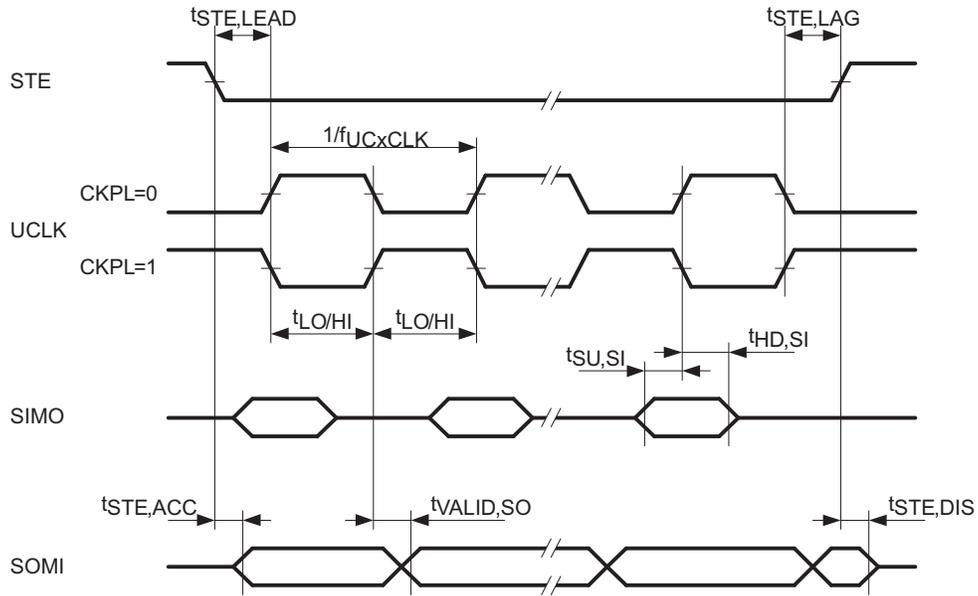
Figure 30. SPI Slave Mode, CKPH = 1
