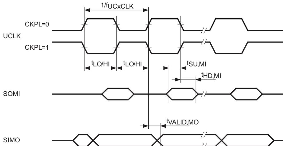
Figure 27. SPI Master Mode, CKPH = 0
