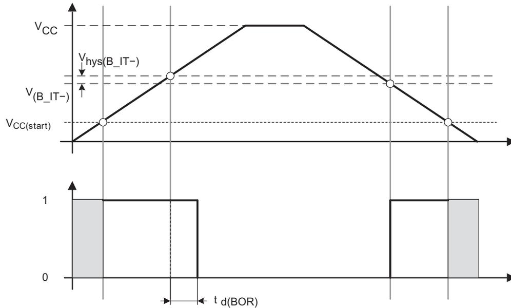
Figure 9. POR/Brownout Reset (BOR) vs Supply Voltage
