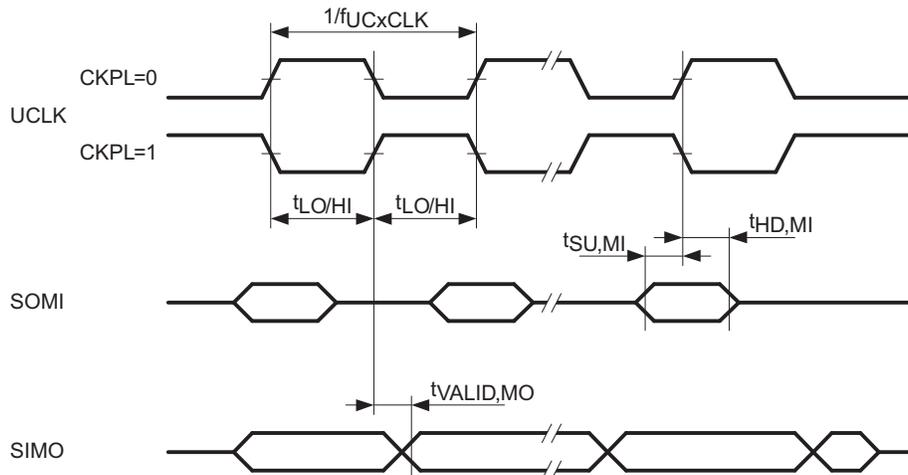
Figure 28. SPI Master Mode, CKPH = 1
