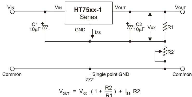
**Circuit for Increasing Output Voltage**
