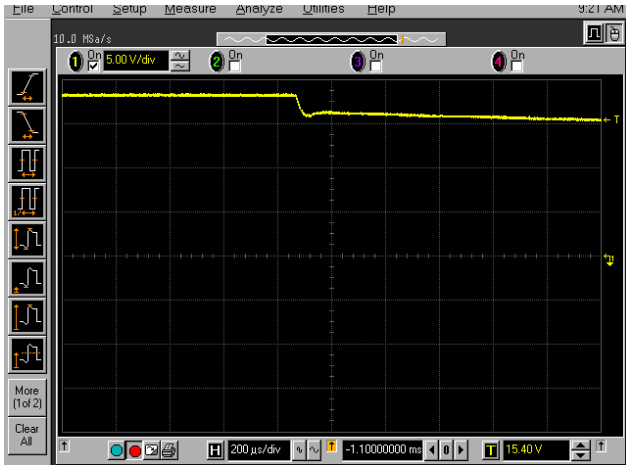
FIGURE 10. VLNB TRANSITIONS FROM 18.3V TO 13.3V
