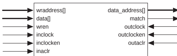
Figure 23. APEX 20KE CAM Block Diagram
