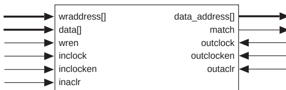
Figure 23. APEX 20KE CAM Block Diagram
