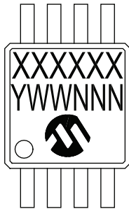
8-Lead MSOP (3x3 mm)
