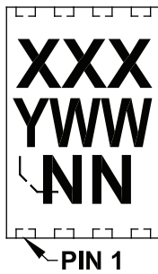
8-Lead DFN (2x3x0.9 mm)
