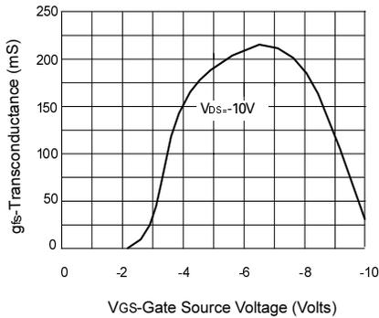
**Transconductance v gate-source voltage**
