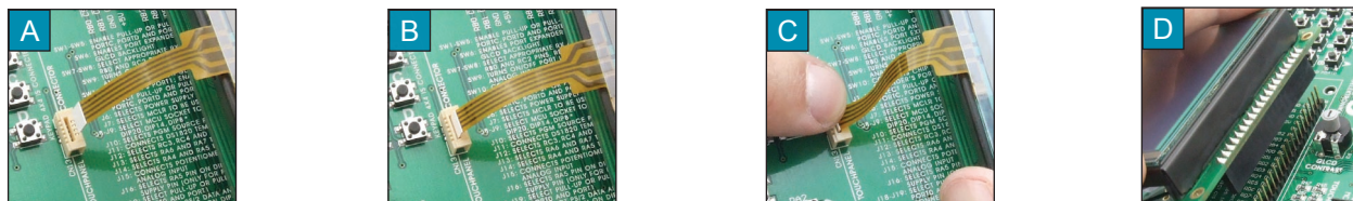
Figure 16-3: Connecting touch panel
