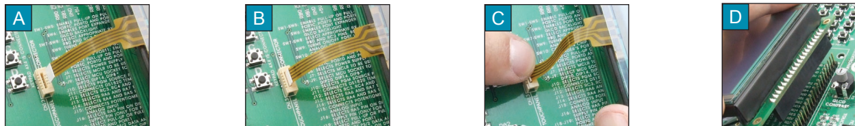
Figure 16-3: Connecting touch panel
