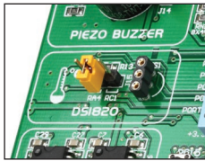
Figure 10-1: DS1820 connector (DS1820 is not connected)
