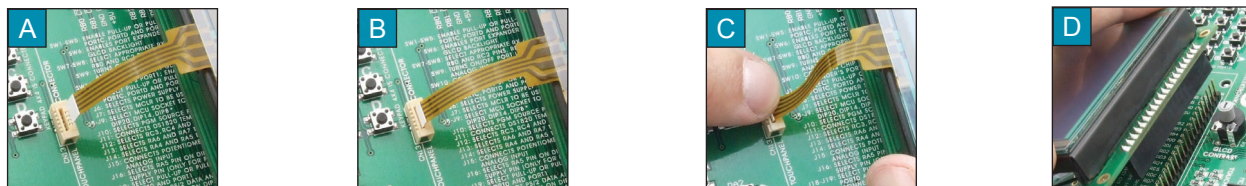
Figure 16-3: Connecting touch panel
