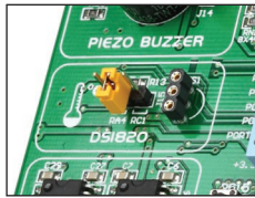
Figure 10-1: DS1820 connector (DS1820 is not connected)
