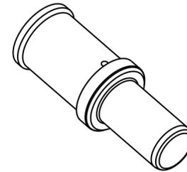
TYPE 3: FOR WIRE GAUGE 50mm<sup>2</sup>, OTHER SPEC. REFER TO TYPE 1 (50mm<sup>2</sup>)
