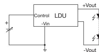
A Control Voltage lower than 0.15 V will turn the output off
