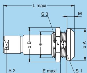
**PSA Fixed socket, nut fixing, cable collet**
