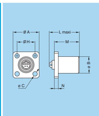
**EBC** Fixed socket with square flange, protruding shell and screw fixing
