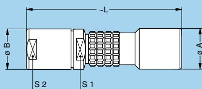
**PHG** Free socket, key (G) or keys (A to C and L), cable collet and oversize cable collet <sup>1)</sup>
