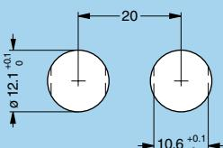
**Note:** mounting nut torque: 4.5 Nm (1N = 0.102 kg)
