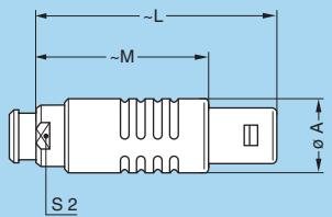
**FFL** Straight plug, cable collet, with PSU and PPSU outer shell, inner anti-rotating device and nut for fitting a bend relief <sup>1)</sup>
