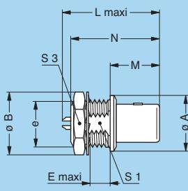
**FAG Fixed plug, non-latching, nut fixing, key (G) or keys (A...M and R)**
