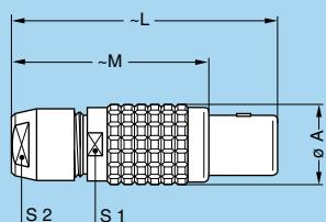
**FFG** Straight plug, non-latching, key (G) or keys (A...M), cable collet
