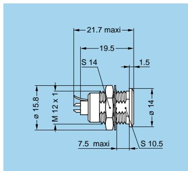
**ERN Fixed socket nut fixing, with earthing tag**
