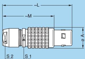
**FGG Straight plug, key (G) or keys (A...M and R), cable collet**
