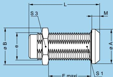
**SWH Fixed coupler, nut fixing, watertight or vacuumtight**
