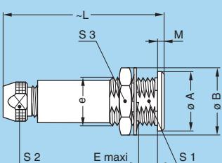
**PSA Fixed socket, nut fixing, cable collet**
