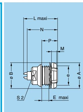
**EFG Fixed socket, nut fixing, key (G) or keys (A...M), with two flats on the shell and O-ring (back panel mounting)**
