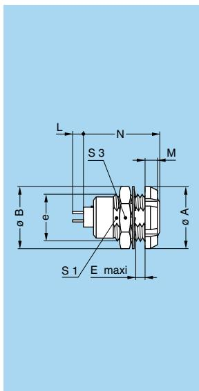
**ECG** Fixed socket with two nuts, key (G) or keys (A...F and R) and straight contact for printed circuit (back panel mounting)
