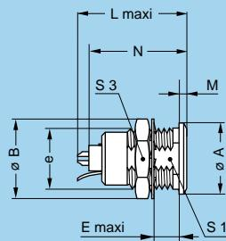
**ENG** Fixed socket with earthing tag, nut fixing, key (G or J), PEEK outer shell
