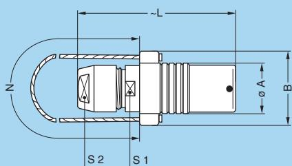
**PNG Free socket, nut fixing, key (G) or keys (A...L and R), cable collet with lanyard release**
