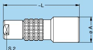
**PCP Free socket, cable collet and inner anti-rotating device**
