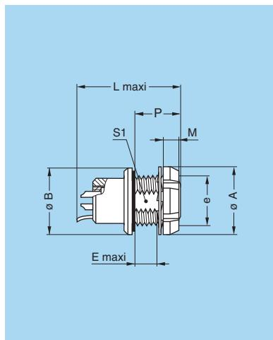
**HMG** Fixed socket with earthing tag, nut fixing, key (G) or keys (A...M), watertight or vacuumtight (back panel mounting)
