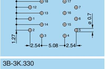
**Elbow socket (90°) for printed circuit (B series)** **P18** **P19** **P20**
