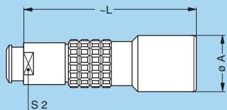
**PHG** Free socket, key (G) or keys (A to F, L and R), cable collet and nut for fitting a bend relief<sup>1)</sup>
