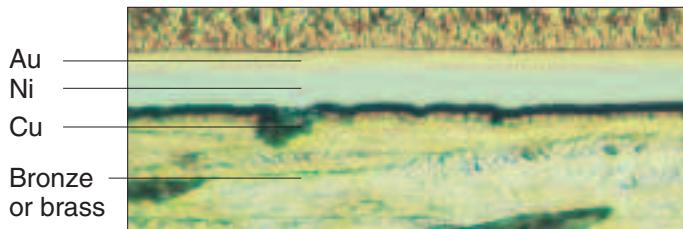
LEMO male solder and print contacts are made of brass (UNS C 38500). Male crimp contacts are made of brass (UNS C 34500) or annealed brass (UNS C 38500) with optimum hardness (HV) for crimping onto the wire.
