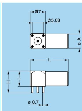
**EPL Elbow (90°) socket for printed circuit**
