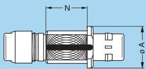
**FIG Straight plug for remote handling, key (G) or keys (A...L and R), special alignment mark, knurled handling surface, cable collet**
