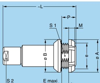
**PEG** Fixed socket, nut fixing, key (G) or keys (A to F, L and R), cable collet (back panel mounting)
