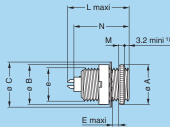
**ESG** Fixed socket with two round nuts, key (G) or keys (B), long threaded shell
