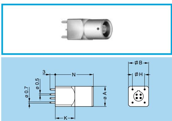
**EZG** Straight socket for printed circuit, key (G) or keys (A, B)
