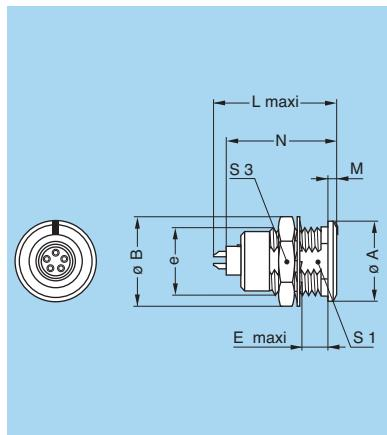
**EKG Fixed socket, nut fixing, key (G) or keys (A...L and R), special alignment mark on the front**
