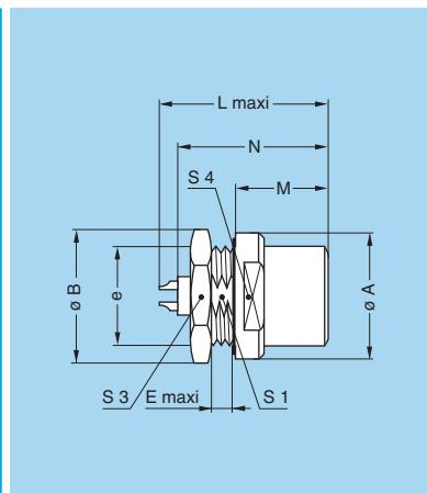
**EHG** Fixed socket, nut fixing, key (G) or keys (A to F and L), protruding shell
