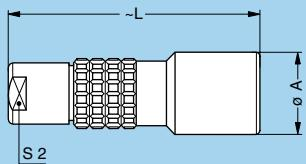
**PHG** Free socket, key (G) or keys (A to C and L), cable collet
