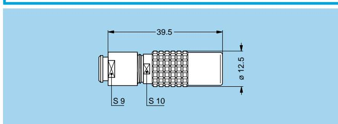
**PCA Free socket, cable collet and nut for fitting a bend relief**
