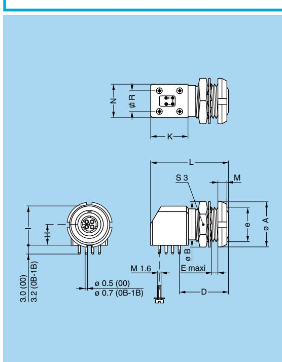
**EXG Elbow (90°) socket for printed circuit with two nuts, key (G) or keys (A...F) (solder or screw fixing) (back panel mounting)**
