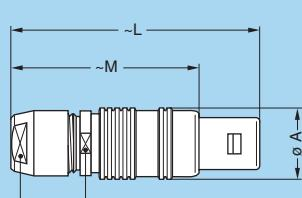
**FFL Straight plug, flats on latch sleeve, cable collet and inner anti-rotating device**
