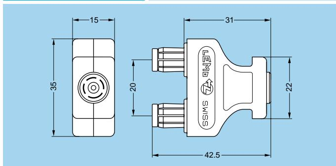
**CFF Bridge plug with two non-latching plugs**
