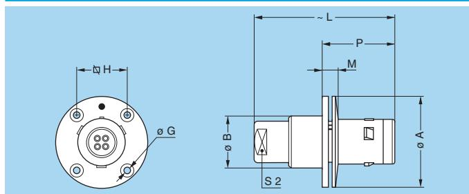
**FXG** Fixed plug with round flange, key (G) or keys (A to F, L and R) and screw fixing
