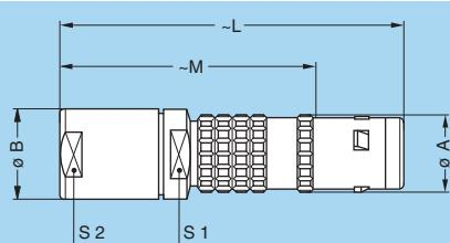
**FGG Straight plug, key (G) or keys (A to C and L), cable collet and oversize cable collet<sup>1)</sup>**
