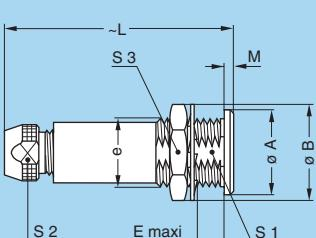
**PSP Fixed socket, nut fixing, cable collet
