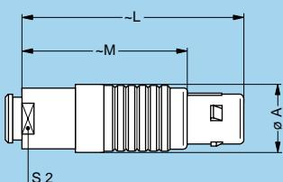
**FGG** Straight plug, key (G or J), cable collet, PEEK outer shell and nut for fitting a bend relief <sup>1)</sup>
