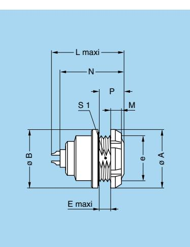
**EEG** Fixed socket, nut fixing, key (G)
