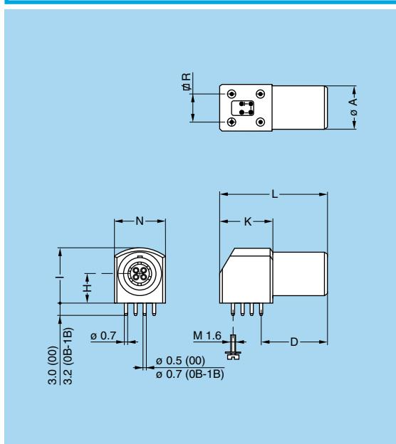
**EPG Elbow (90°) socket for printed circuit, key (G) or keys (A...F) (solder or screw fixing)**
