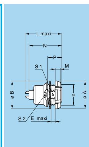
**EEG Fixed socket, nut fixing, key (G) or keys (A...M and R) (back panel mounting)**
