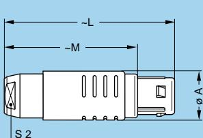
**FGY** Straight plug, keys (Y), cable collet and PSU or PPSU outer shell
