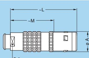
**FGG Straight plug, key (G) or keys (A to C and L), cable collet and nut for fitting a bend relief<sup>1)</sup>**
