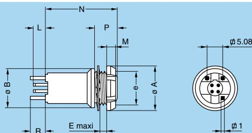
**XPF Fixed socket, nut fixing, long shell, keys (F) for printed circuit (back panel mounting)**
