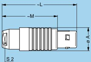
**FGG** Straight plug, key (G or J), cable collet, PEEK outer shell
