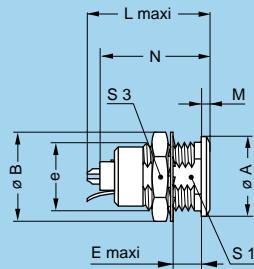
**ENY** Fixed socket with earthing tag, nut fixing, keys (Y), PSU or PPSU outer shell
