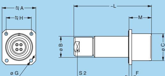
**PBG** Fixed socket, key (G) with square flange, cable collet and screw fixing
