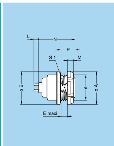
**EEG Fixed socket, nut fixing, key (G) or keys (A to F and R) with straight print contacts for printed circuit (back panel mounting)**
