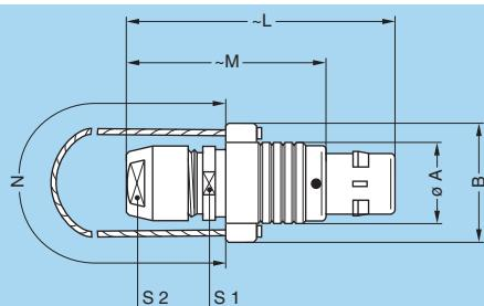
**FNG** Straight plug, key (G) or keys (A...M and R), cable collet and lanyard release
