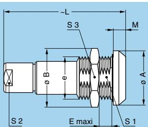
**PKG** Fixed socket, nut fixing, key (G) or keys (A to C and L), cable collet
