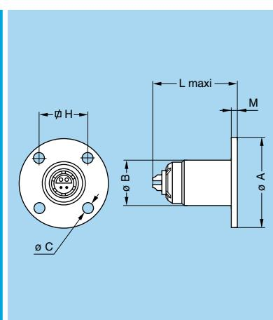
**EBS** Fixed socket with round flange and screw fixing
