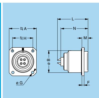
**EBG Fixed socket with square flange, key (G) or keys (A to F, L and R) and screw fixing**
