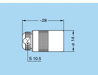
**PHG.2G Free socket, key (G), cable collet and nut for fitting a bend relief<sup>1)</sup>**
