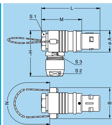
**FMG** Elbow (90°) plug, key (G) or keys (A...M), cable collet and lanyard release, long key <sup>1)</sup>
