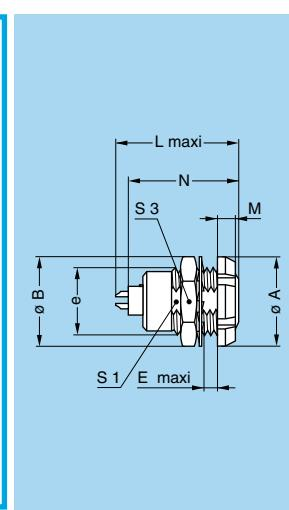
**ECG Fixed socket with two nuts, key (G) or keys (A...M and R) (back panel mounting)**
