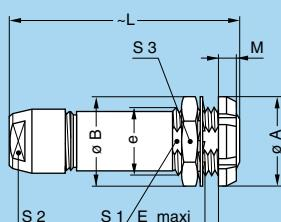
**PFG Fixed socket, with two nuts, key (G) or keys (A...M and R), cable collet (back panel mounting)**
