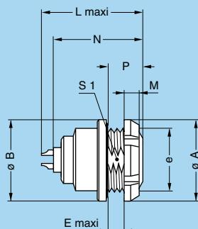
**EEG** Fixed socket, nut fixing, key (G)
