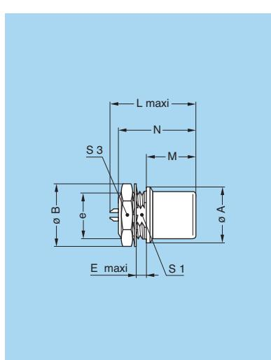
**EHG Fixed socket, nut fixing, key (G) or keys (A...M and R), and protruding shell**
