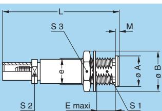
**PSS Free socket, nut fixing for cable crimping**
