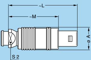
**FFP** Straight plug, cable collet, PEEK or POM outer shell, inner anti-rotating device and nut for fitting a bend relief <sup>1)</sup>
