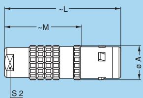
**FGG Straight plug, key (G) or keys (A to C and L), cable collet**
