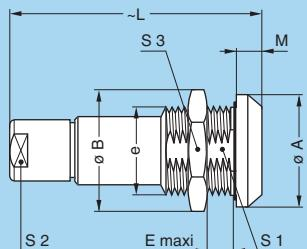
**PKG** Fixed socket, nut fixing, key (G) or keys (A to F, L and R), cable collet
