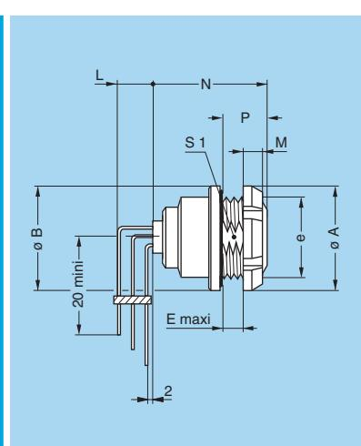
**EEG Fixed socket, nut fixing, key (G) or keys (A to F and R) with elbow (90°) contacts for printed circuit (back panel mounting)**
