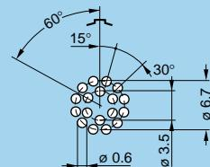
**Note:** mounting nut torque: 6 Nm (1N = 0.102 kg)
