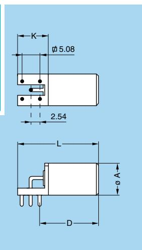
**EPL Elbow (90°) socket for printed circuit**
