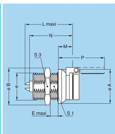
**EVG** Fixed socket, nut fixing, key (G) or keys (A to F and L) and dust cap (spring loaded)
