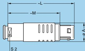
**FGY** Straight plug, keys (Y), cable collet and PSU or PPSU outer shell and nut for fitting a bend relief<sup>1)</sup>
