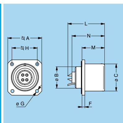
**EDG Fixed socket with square flange, key (G) or keys (A to F, L and R), protruding shell and earthing tag, screw fixing**
