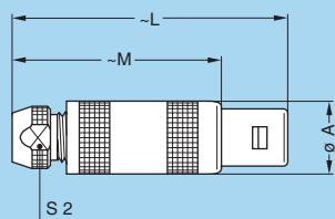
**FFP Straight plug, cable collet and inner anti-rotating device**
