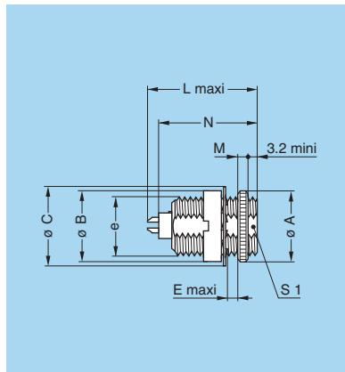
**ESG Fixed socket with two round nuts, key (G) or keys (A...L), long threaded shell (back panel mounting)**
