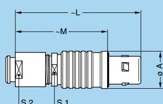
**FEG** Straight plug, key (G) or keys (A...L), cable collet, front seal and nut for fitting a bend relief <sup>1)</sup> (IP 54 protection index when mated)
