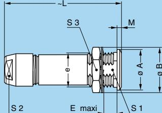
**PKG Fixed socket, nut fixing, key (G) or keys (A...M and R), cable collet**
