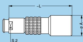
**PHG** Free socket, key (G) or keys (A to C and L), cable collet and nut for fitting a bend relief <sup>1)</sup>
