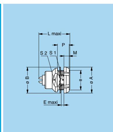
**EEP** Fixed socket, nut fixing (back panel mounting)
