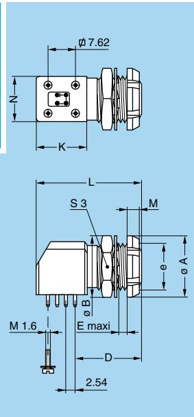
**EXP Elbow (90°) socket for printed circuit with two nuts
