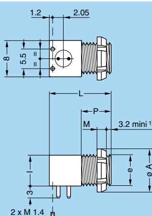
**XRB** Elbow (90°) socket for printed circuit, keys (B),
