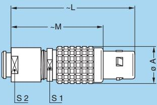
**FGG Straight plug, key (G) or keys (A...M), cable collet and nut for fitting a bend relief<sup>2)</sup>**
