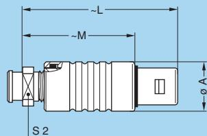
**FFE Straight plug, cable collet, front seal and nut for fitting a bend relief <sup>1)</sup> (protected to IP54 when mated)**
