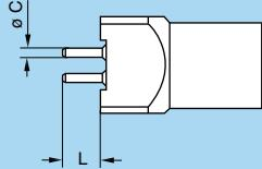
Note: Mounting torque for screws: 0.1 Nm.
