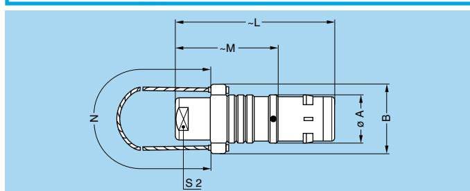
**FNG** Straight plug, key (G) or keys (A to F and L), cable collet and lanyard release
