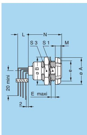
**ECG** Fixed socket with two nuts, key (G) or keys (A...F) with elbow (90°) contact for printed circuit (back panel mounting)
