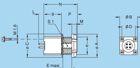
**EYG Fixed socket for printed circuit, nut fixing, key (G) or keys (A...F) (back panel mounting)**
