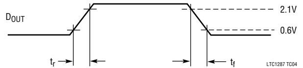
Voltage Waveforms for DOUT Rise and Fall Times, t r , t f
