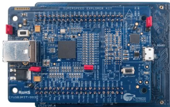
2. Plug the HSMC Interconnect Board (CYUSB3ACC-006) into the Altera® FPGA board (The Altera FPGA board is not part of this kit)
