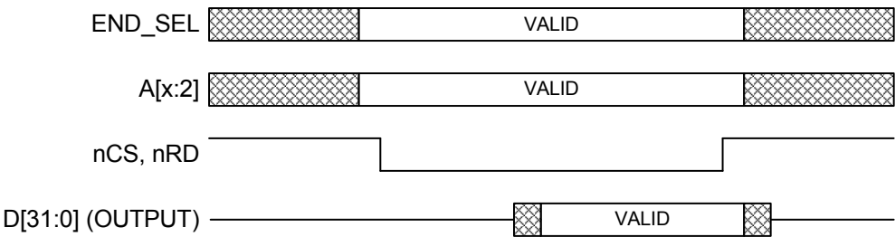
Figure 8.3 Functional Timing for PIO Read Operation
