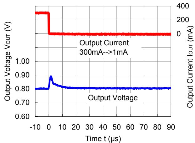
**RP504x081x ( $V_{IN} = 3.6$  V)**
