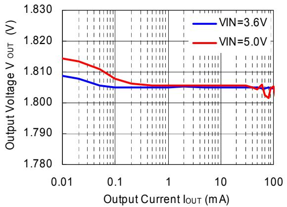
**RP504x  $V_{OUT} = 1.8 \text{ V}$**
