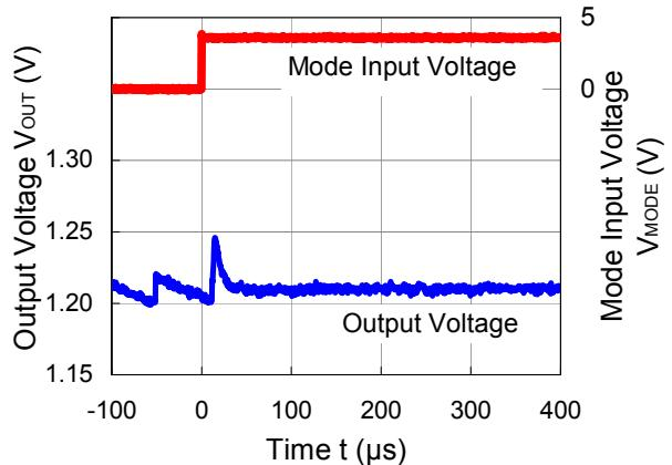
**RP504x ( $V_{OUT} = 1.2$  V,  $I_{OUT} = 1$  mA)**
