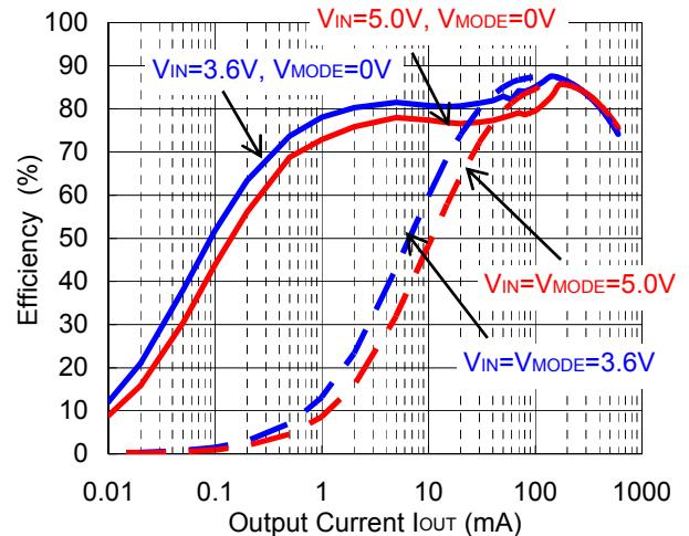
RP504x  $V_{OUT} = 1.8$  V
