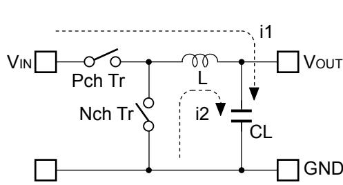
**Figure 1. Basic Circuit**
