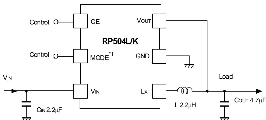
\*<sup>1</sup> MODE = "H": forced PWM control, MODE = "L": PWM/VFM auto switching control
