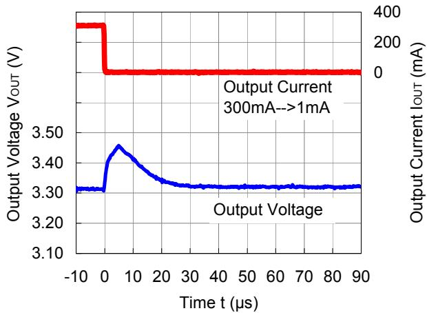
**RP504x331x ( $V_{IN} = 5.0$  V)**
