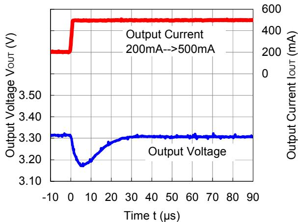
**RP504x331x ( $V_{IN} = 5.0$  V)**
