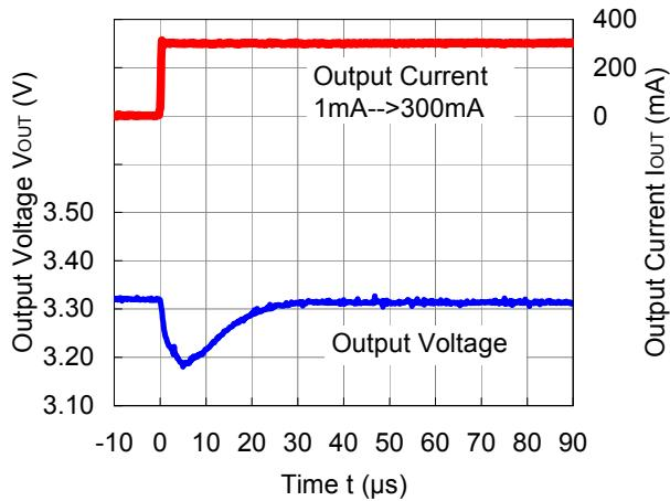
**RP504x331x ( $V_{IN} = 5.0$  V)**
