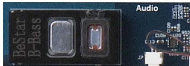
A BeStar B-Bass 1-W speaker is driven by a [WM9001 1W Dual-Mode Class AB/D Speaker Driver](#) operated in Class D mode. The input to the WM9001 is AC-coupled from the 12-bit DAC channel 0 of the Synergy S7G2 MCU. A GPIO is used to enable the amplifier, saving power if/when audio output is not required:
