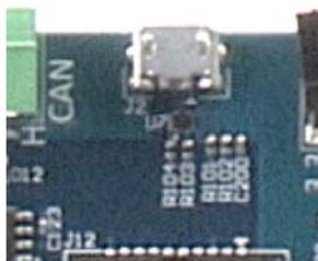
The Synergy S7G2 MCU features independent USB 2.0 Host and USB 2.0 Device (or “function”) ports; the Host port capable of High Speed 480mbps data rates, the Device port limited to Full Speed 12mbps.
