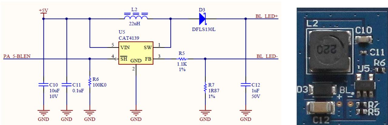
A PWM-capable MCU port bit is connected to this controller's **SH#** (shutdown) pin:
