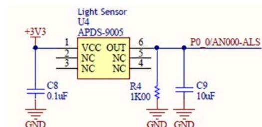
3.3 V on an Analog to Digital Converter (ADC) input on the MCU. Software can poll this ADC periodically. The ALS is connected as follows:
