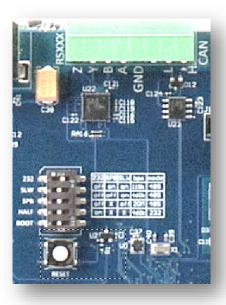
The large green 3.5-mm connector J10 delivers RS232, RS422, or RS485 as well as high performance CAN to external industrial networks. A screw terminal plug is supplied, enabling easy wiring of termination or daisy chained cabling. The connector's signals are clearly marked on the PCB as follows:
