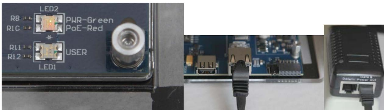
Alternatively, use the small barrel jack adapter cable and your own 2.1-mm positive-center 5-V barrel jack power supply to power the PE-HMI1 directly. When the 5-V direct power input is present and active, the LED1 power indicator will be GREEN.
