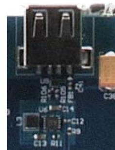
**R13** sets the current limit: in this design 51.0kΩ indicates a limit of ~500mA. At currents above this limit, the voltage on the output to the connector drops precipitously to limit the current to this maximum. The **FAULT#** open drain output from the chip indicates when the chip is in current-limiting mode and can be used by software to detect this fault condition.
