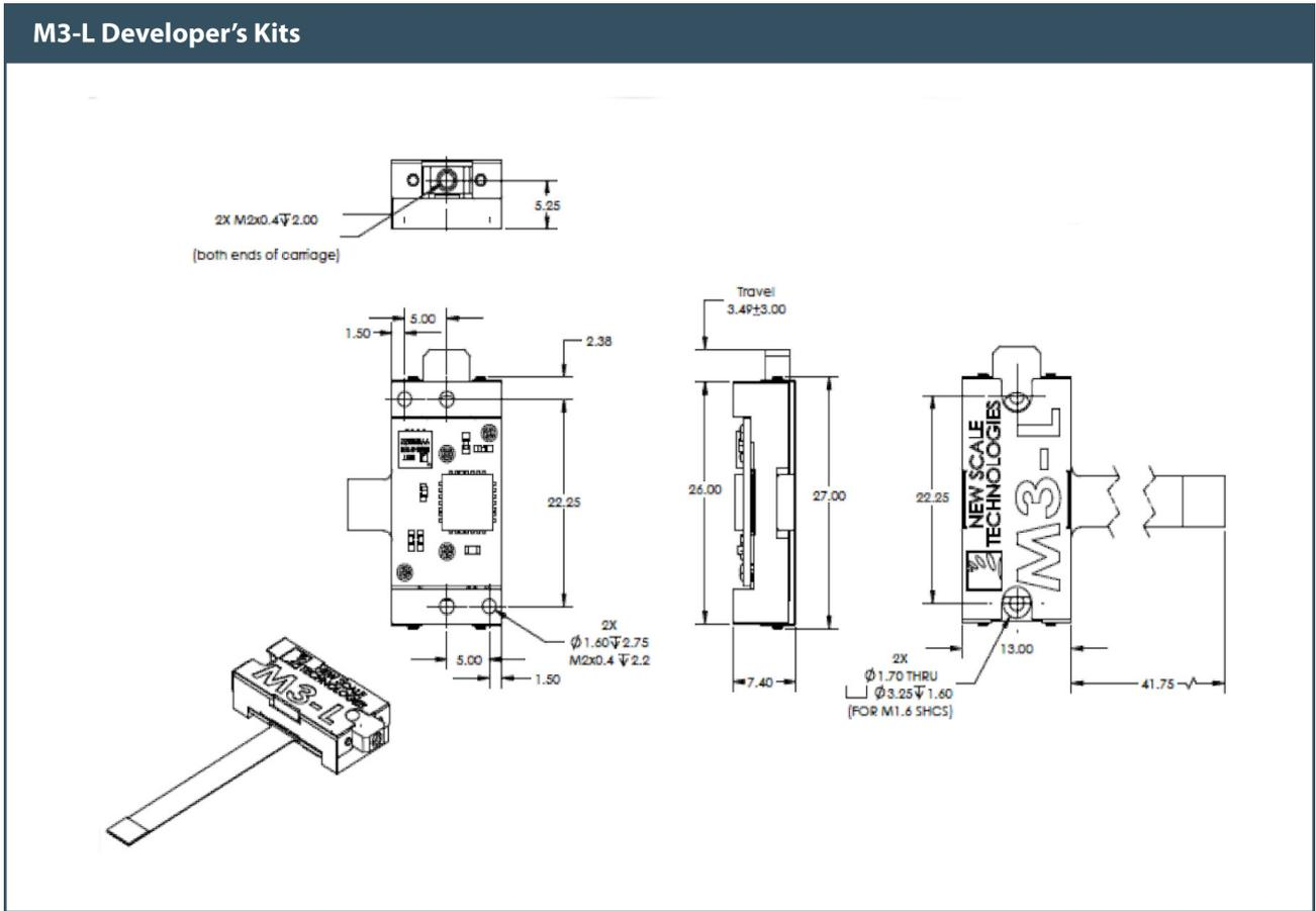
M3-L Developer's Kits allow OEMs to rapidly integrate miniature, high resolution linear motion controls with up to 6 mm total travel. Kits include one M3-L module, USB control stick with SPI output, and New Scale Pathway™ software.
