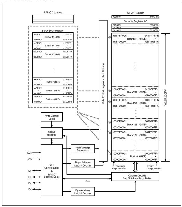
Figure 2. W25R256JV Serial Flash Memory Block Diagram
