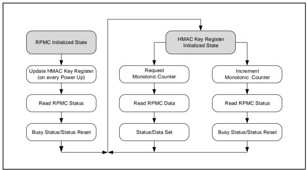
Figure 3b. W25R256JV RPMC Operation Flow Diagram
