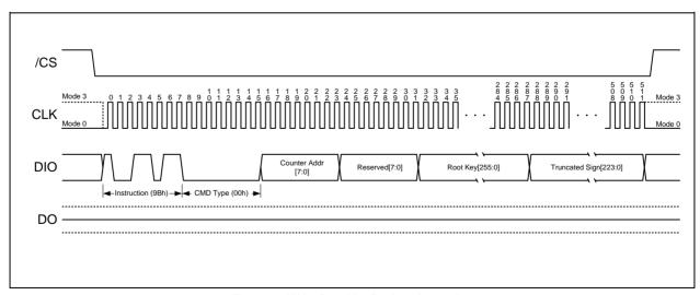
Figure 43. Write Root Key Register Instruction
