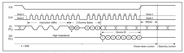
Figure 38c. Release Power-down / Device ID Instruction
