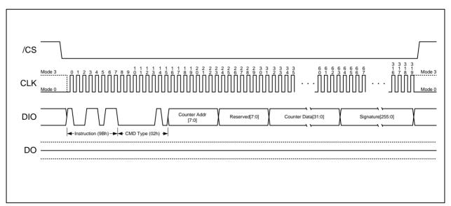
Figure 45. Increment Monotonic counters Instruction
