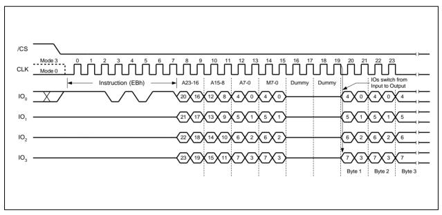
Figure 24a. Fast Read Quad I/O Instruction (Initial instruction or previous M5-4≠10)
