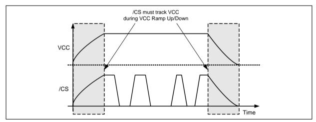
Figure 58b. Power-up, Power-Down Requirement
