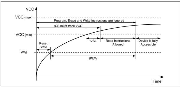
Figure 58. Power-up Timing and Voltage Levels
