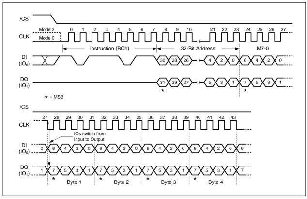
Figure 23a. Fast Read Dual I/O with 4-Byte Address Instruction (Initial instruction or previous M5-4  $\neq$  10)
