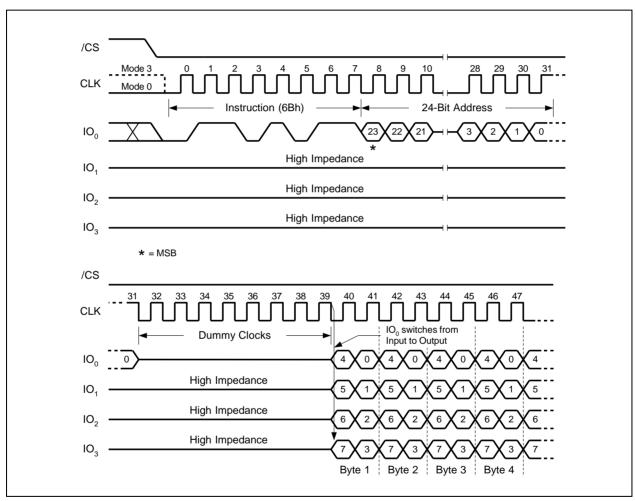
Figure 20. Fast Read Quad Output Instruction
