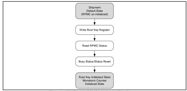
Figure 3a. W25R256JV RPMC Initialization Flow Diagram
