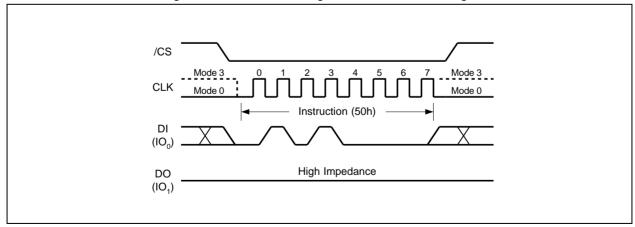
Figure 7. Write Enable for Volatile Status Register Instruction
