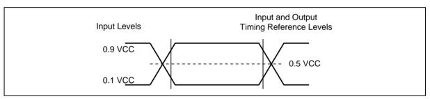
Figure 59. AC Measurement I/O Waveform
