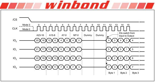
Figure 24b. Fast Read Quad I/O Instruction (Previous instruction set M5-4 = 10) 32-Bit Address is required when the device is operating in 4-Byte Address Mode
