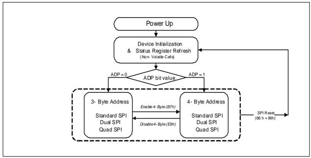
Figure 3. W25R256JV Serial Flash Memory Operation Diagram
