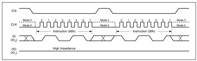
Figure 57a. Enable Reset and Reset Instruction Sequence
