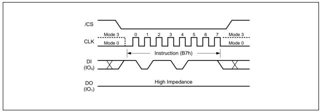
Figure 12. Enter 4-Byte Address Mode instruction
