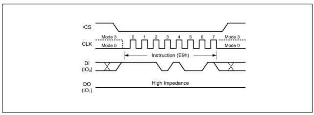
Figure 13. Exit 4-Byte Address Mode instruction
