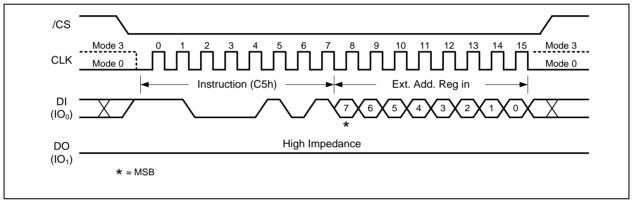
Figure 11a. Write Extended Address Register Instruction
