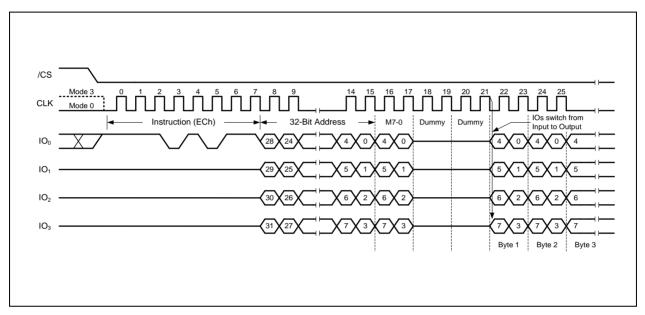
Figure 25a. Fast Read Quad I/O with 4-Byte Address Instruction (Initial instruction or previous M5-4≠10)
