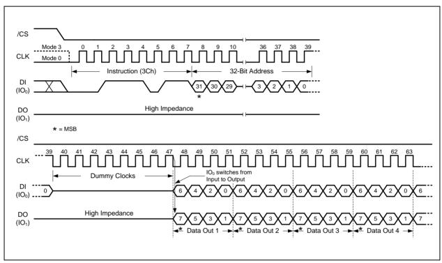
Figure 19. Fast Read Dual Output with 4-Byte Address Instruction
