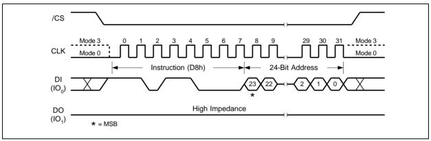
Figure 33a. 64KB Block Erase Instruction 32-Bit Address is required when the device is operating in 4-Byte Address Mode
