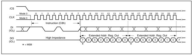
Figure 10a. Read Extended Address Register Instruction
