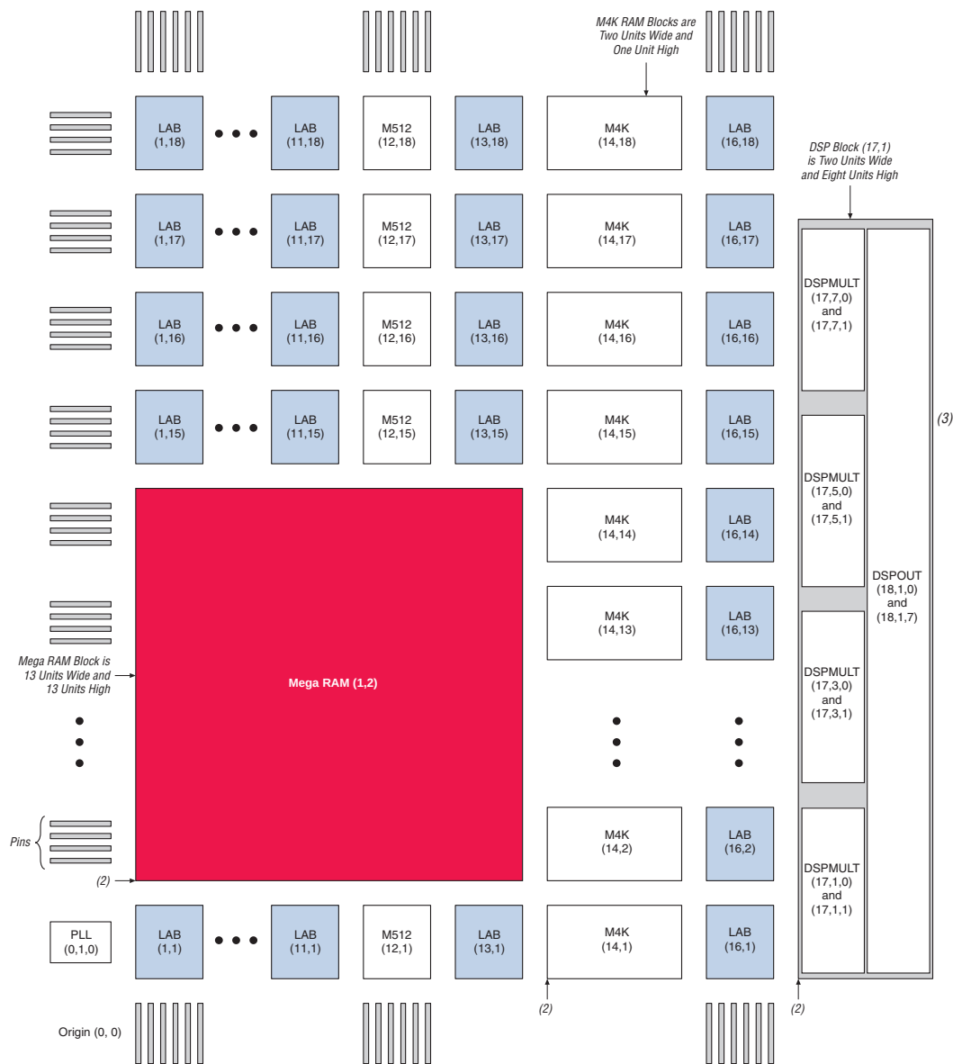
Figure 10–2. Stratix & Stratix GX Architectural Elements Note (1)
