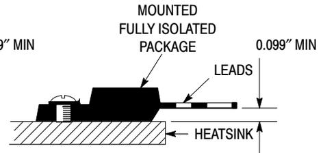
Figure 22c. Screw Mounting Position for Isolation Test Number 3
