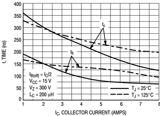
Figure 11. Inductive Switching,  $t_c$  and  $t_{fi}$
