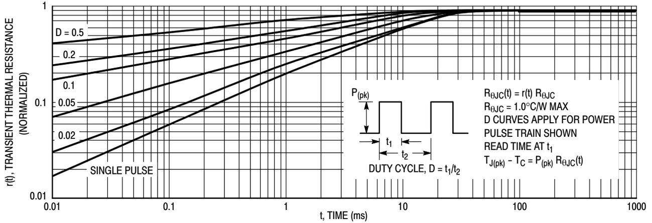
Figure 20. Typical Thermal Response ( $Z_{\theta_{JC}}(t)$ ) for MJE18008
