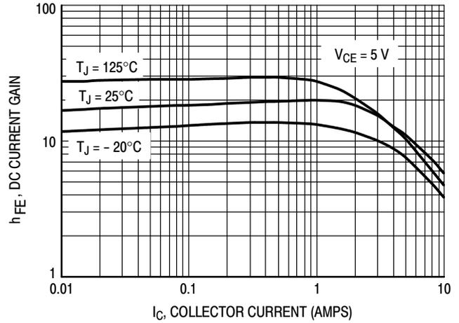
Figure 2. DC Current Gain @ 5 Volts
