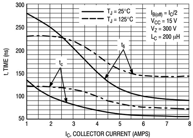
Figure 12. Inductive Switching,  $t_c$  and  $t_{fi}$
