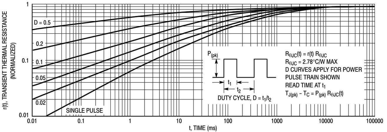
Figure 21. Typical Thermal Response ( $Z_{\theta_{JC}}(t)$ ) for MJF18008
