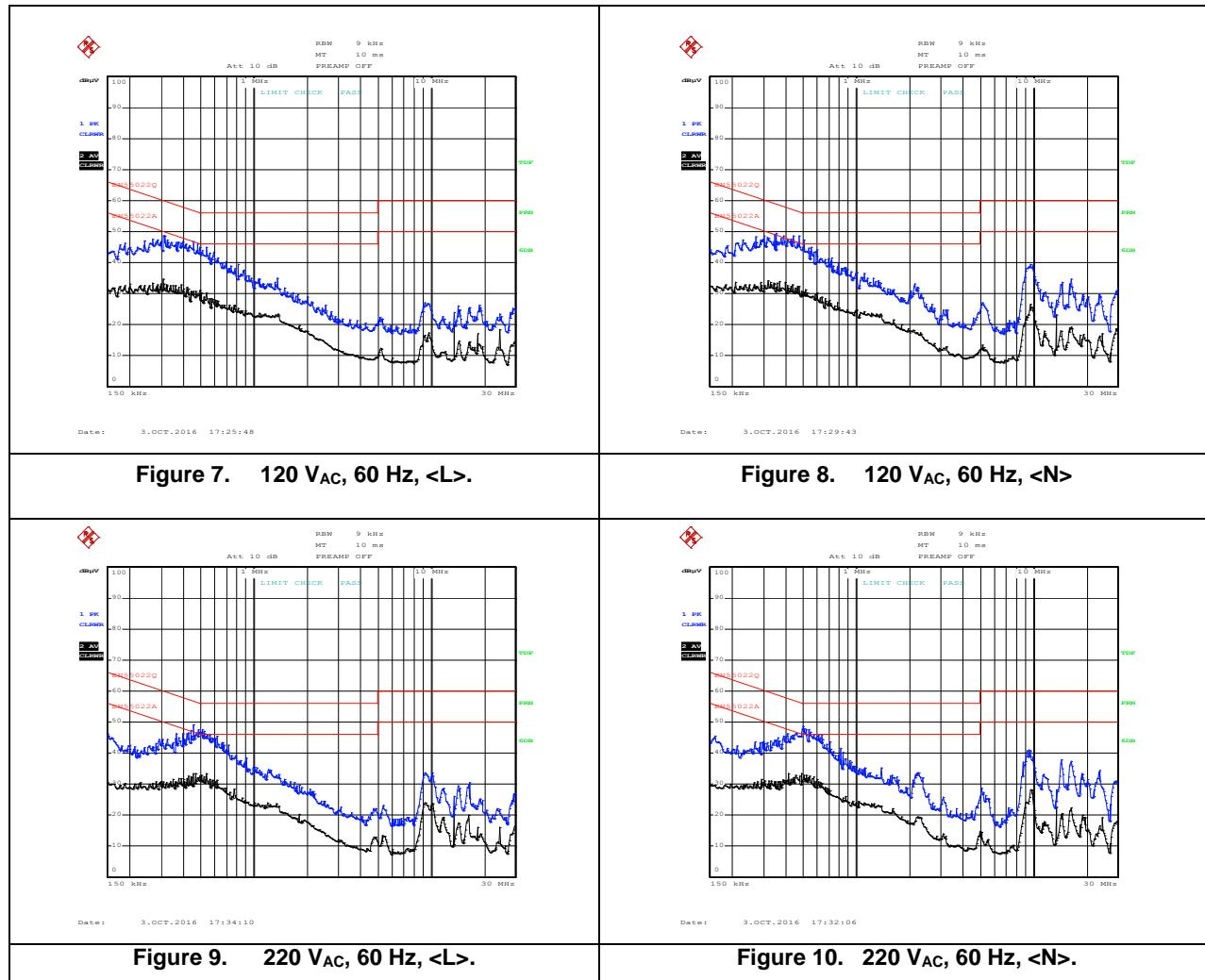
All measurements were conducted in observance of EN55022 criteria.
