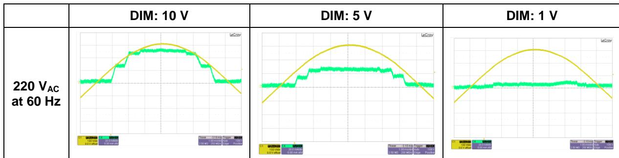
**Figure 6. Ch1: V<sub>IN.ac</sub>, 100 V/div, Ch4: I<sub>IN.ac</sub> 20.0 mA/div**
