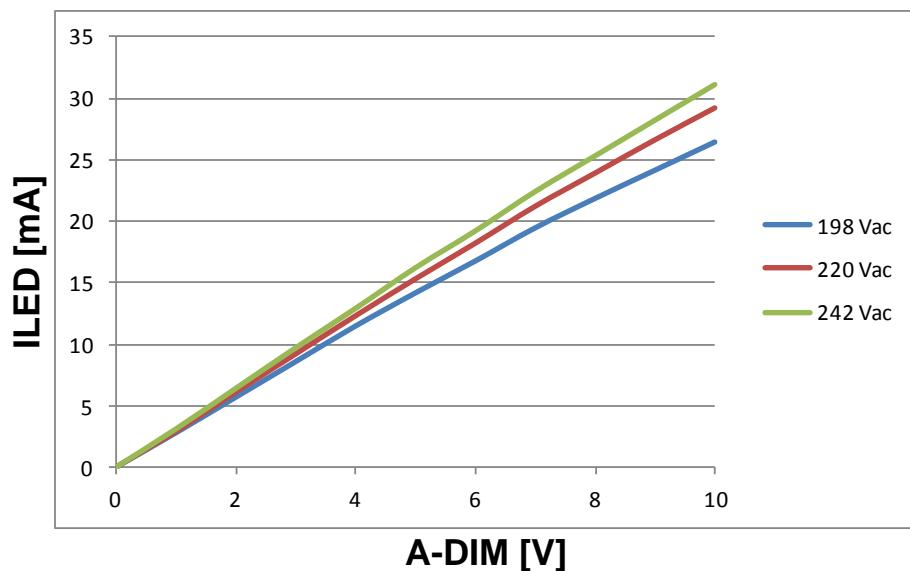
FL77905 analog dimming function can be implemented with a few external components.
