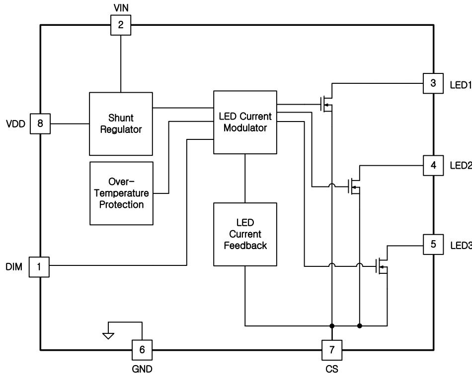
Figure 1. Simplified FL77904 Block Diagram
