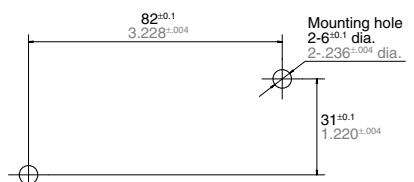
**Dimension:**Less than 10mm .394inch:  $\pm 0.3 \pm 0.012$ 10 to 50mm .394 to 1.969inch:  $\pm 0.6 \pm 0.024$ Min. 50mm 1.969 inch:  $\pm 1.0 \pm 0.039$ **General tolerance**
