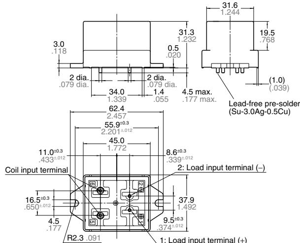
**Schematic (Bottom view)**
