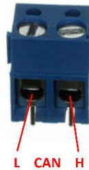
Figure 43: CAN1 Terminal Block
