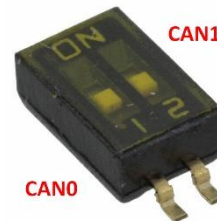
Figure 44: CAN Termination Switch
