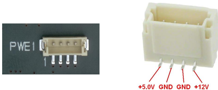
Figure 35: Power Connector PWE1
