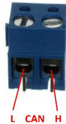
Figure 43: CAN1 Terminal Block
