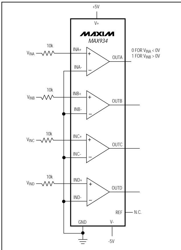
Figure 8. Level Shifter:  $\pm 5\text{V}$  Input to CMOS Output
