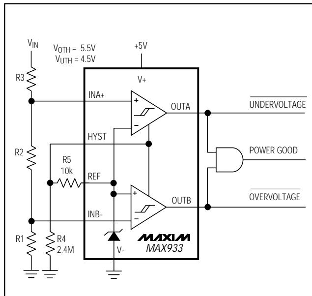
Figure 6. Window Detector
