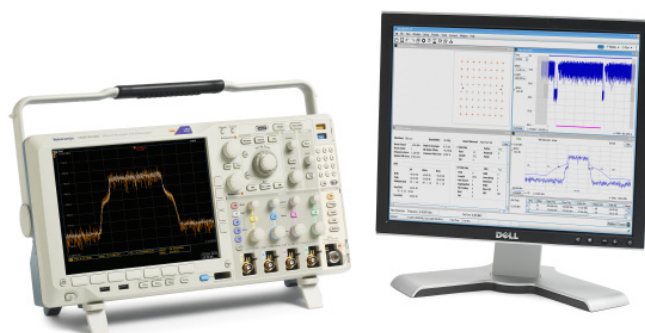
MDO4000C paired with SignalVu-PC to analyze 802.11ac modulation.
