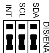
FIG 1: Pulled-up R enable
