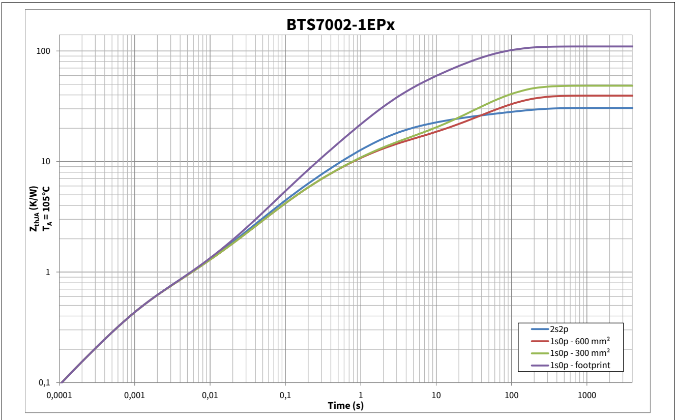
Figure 9 Typical Thermal Impedance. PCB setup according Chapter 4.4.1
