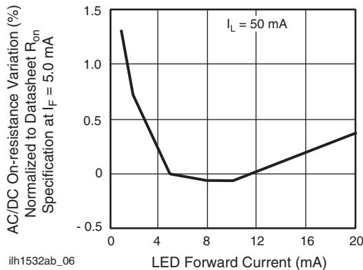
Fig. 7 - Variation in On-Resistance vs. LED Current
