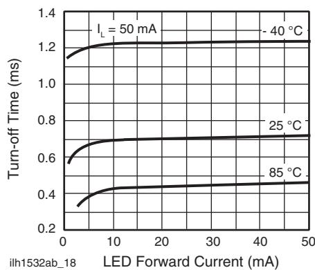
Fig. 19 - Turn-off Time vs. LED Current
