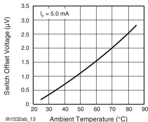
Fig. 14 - Switch Offset Voltage vs. Temperature
