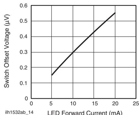
Fig. 15 - Switch Offset Voltage vs. LED Current
