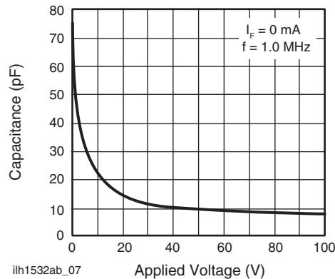
Fig. 8 - Switch Capacitance vs. Applied Voltage
