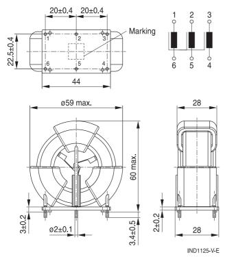
Tolerances to ISO 2768-cl / ISO 8015. Size ISO 14405 (E) All dimensions in mm
