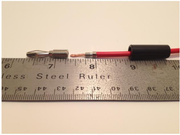
For an 18 awg wire you will need to strip the item back 5/8". Push the wire into the assembly hold the small nut against the insulation and screw it into the banana. Finally pull the insulating cover over the banana and screw in. If your using a smaller gauge wire, you will need to increase your strip length.
