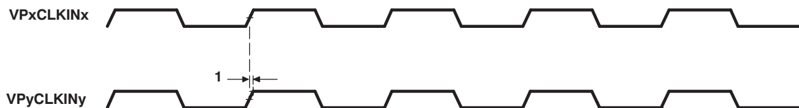
Figure 6-25. Video Port Dual-Display Sync Timing
