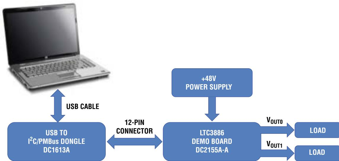
Figure 3. Demo Setup with PC for DC2155A-A
