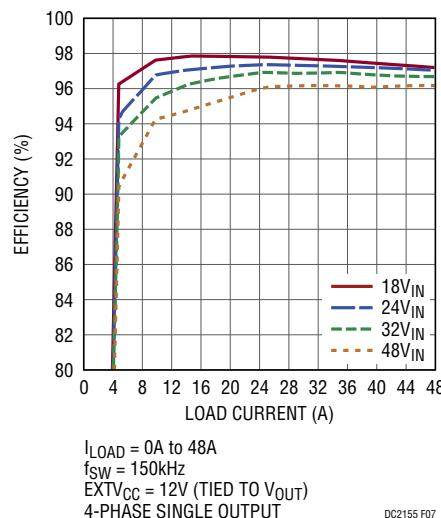
Figure 7. DC2155A-B: Efficiency at 12V<sub>OUT</sub>
