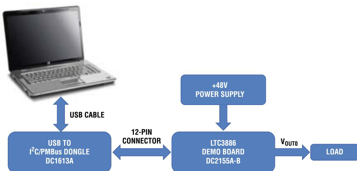
Figure 4. Demo Setup with PC for DC2155A-B
