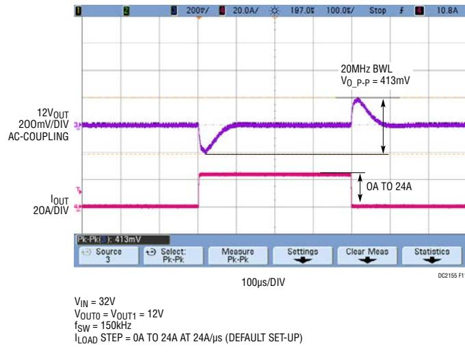
Figure 11. DC2155A-B Load Step Response  $V_{IN} = 32V$
