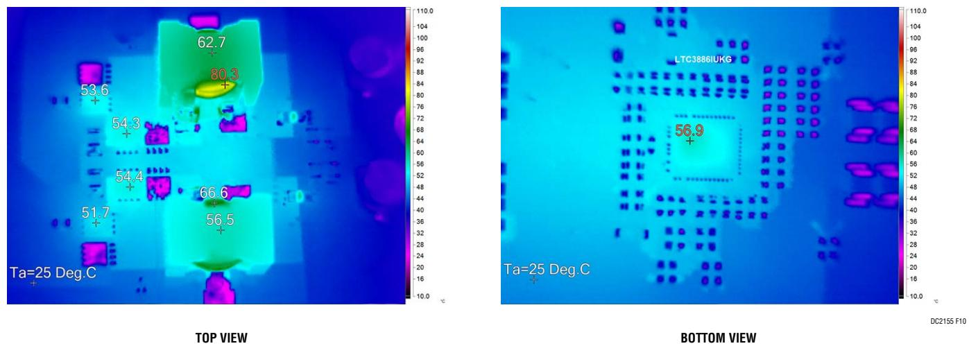
Figure 10. DC2155A-A Thermal Performance
