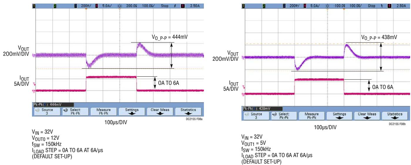
Figure 8. DC2155A-A Load Step Response
