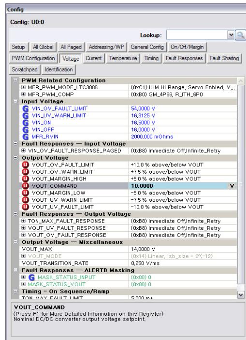
Then, click the "W" (PC to RAM) icon to write these register values to the LTC3886. After finishing this step, you will see the output voltage will change to 10V.
