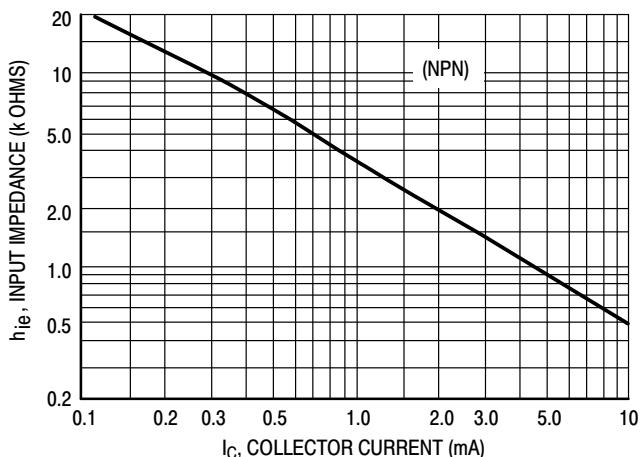
Figure 12. Input Impedance
