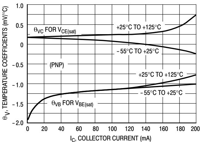
Figure 33. Temperature Coefficients
