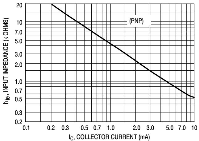
Figure 28. Input Impedance
