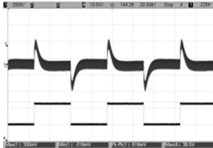
Step Load Transient Response ( V_{in}=48V , V_{out}=nom , C_{load}=470\mu F , I_{out}=50-75-50\% of full load, T_a=+25^{\circ}C )
