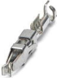
Female contact, is inserted into the plug after crimping the conductor, for the module plug housing MCC 1...-STZ-3,81 and MCC 1...-STZF-3,81, for cross sections of 0.2 mm<sup>2</sup> to 0.34 mm<sup>2</sup>
