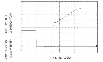
Figure 5. Typical Start-up Using On/Off Voltage ( $I_0 = I_{0,max}$ ).
