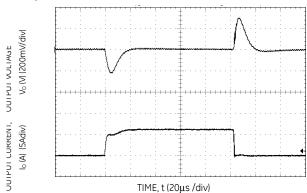
Figure 10. Transient Response to Dynamic Load Change from 0% to 50% to 0% with  $V_{\text{IN}}$ =5V.
