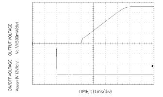
Figure 17. Typical Start-up Using On/Off Voltage (Io = Io,max).
