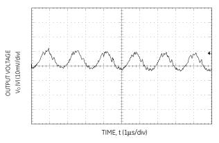
Figure 27. Typical output ripple and noise ( $V_{IN} = 5V$ ,  $I_0 = I_{0,max}$ ).
