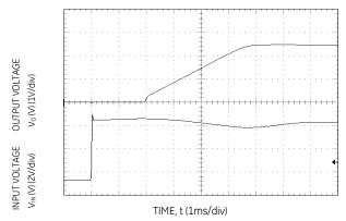
Figure 24. Typical Start-up Using Input Voltage ( $V_{IN} = 5V$ ,  $I_0 = I_{0,max}$ ).
