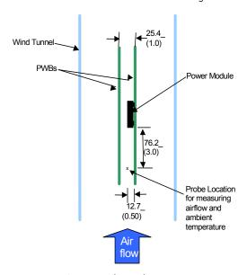
Figure 45. Thermal Test Setup.
