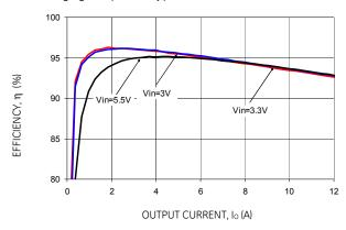
Figure 19. Converter Efficiency versus Output Current.
