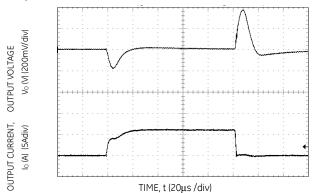
Figure 4. Transient Response to Dynamic Load Change from 0% to 50% to 0% with  $V_{\text{IN}}{=}5V$ .
