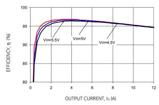
Figure 25. Converter Efficiency versus Output Current.
