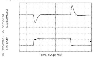
Figure 16. Transient Response to Dynamic Load Change from 0% to 50% to 0% with  $V_{\text{IN}}$ =5V.
