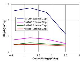
Figure 37. Output ripple voltage for various output voltages with external 1x10  $\mu$ F, 1x47  $\mu$ F, 2x47  $\mu$ F or 4x47  $\mu$ F ceramic capacitors at the output (12A load). Input voltage is 3.3V.
