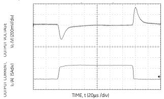
Figure 28. Transient Response to Dynamic Load Change from 0% 50% to 0% with  $V_{\text{IN}}$ =5V.
