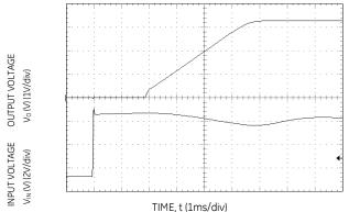
Figure 30. Typical Start-up Using Input Voltage ( $V_{IN} = 5V$ ,  $I_0 = I_{0,max}$ ).
