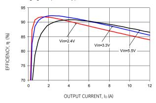
Figure 7. Converter Efficiency versus Output Current.
