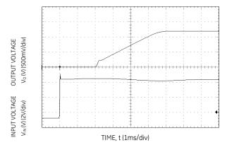
Figure 12. Typical Start-up Using Input Voltage ( $V_{IN} = 5V$ ,  $I_0 = I_{o,max}$ ).
