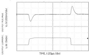
Figure 22. Transient Response to Dynamic Load Change from 0% to 50% to 0% with  $V_{\rm IN}$ =5V.
