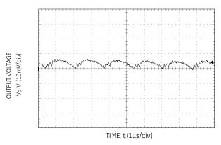
Figure 3. Typical output ripple and noise ( $V_{IN} = 5V$ ,  $I_0 = I_{O,max}$ ).
