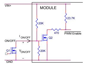
Figure 38. Circuit configuration for using positive On/Off logic.
