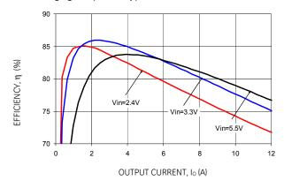
Figure 1. Converter Efficiency versus Output Current.
