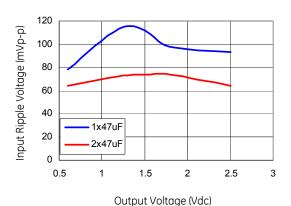
Figure 35. Input ripple voltage in mV, p-p for various output voltages with 1x47  $\mu$ F or 2x47  $\mu$ F ceramic capacitors at the input (12A load). Input voltage is 3.3V.
