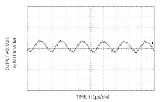
Figure 15. Typical output ripple and noise ( $V_{IN} = 5V$ ,  $I_0 = I_{O,max}$ ).
