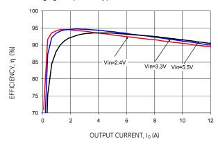
Figure 13. Converter Efficiency versus Output Current.
