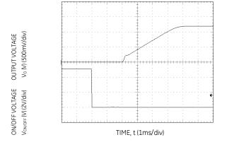
Figure 11. Typical Start-up Using On/Off Voltage ( $I_0 = I_{o,max}$ ).
