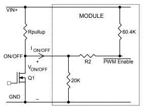
Figure 39. Circuit configuration for using negative On/Off logic.
