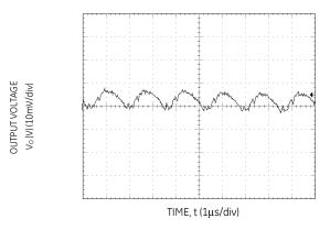
Figure 9. Typical output ripple and noise ( $V_{IN} = 5V$ ,  $I_0 = I_{0,max}$ ).
