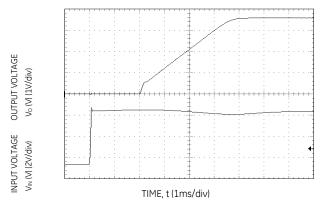
Figure 18. Typical Start-up Using Input Voltage ( $V_{IN} = 5V$ ,  $I_0 = I_{0,max}$ ).
