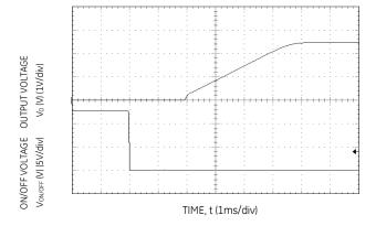
Figure 23. Typical Start-up Using On/Off Voltage ( $I_0 = I_{0,max}$ ).
