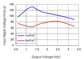
Figure 34. Input ripple voltage for various output voltages with 1x47  $\mu$ F or 2x47  $\mu$ F ceramic capacitors at the input (12A load). Input voltage is 5V.
