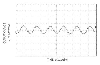
Figure 21. Typical output ripple and noise ( $V_{IN} = 5V$ ,  $I_0 = I_{0,max}$ ).
