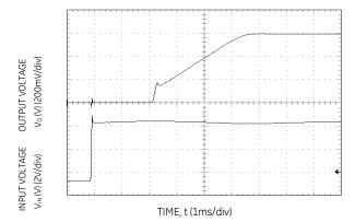
Figure 6. Typical Start-up Using Input Voltage ( $V_{IN} = 5V$ ,  $I_0 = I_{0,max}$ ).
