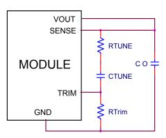
Figure. 44. Circuit diagram showing connection of  $R_{\text{TUME}}$  and  $C_{\text{TUNE}}$  to tune the control loop of the module.
